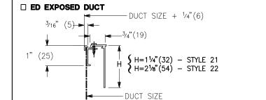
ED APPLICATION IS SUPPLIED COMPLETE WITH BORDER AND DUCT MOUNTING FRAME
